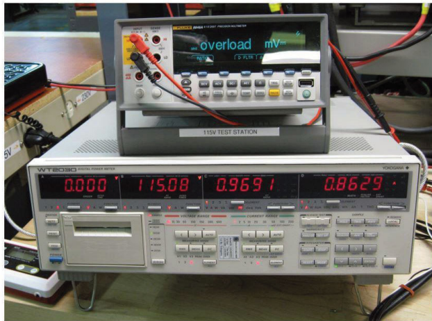
The Yokogawa WT-2030 captures input power readings, including input voltage, input current, input frequency, and input power. It also measures power factor, total harmonic distortion, and output current.
